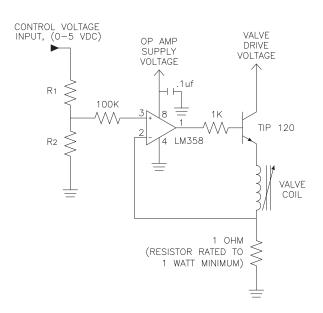
This simple current driver circuit draws only 1 mA at the input control (0-5VDC) and provides control for any LM-Pro valve configuration regardless of valve voltage or resistance.
